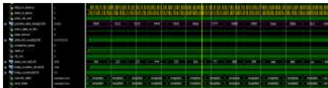
Figure 13: Simulated output for encoded data sent to ARINC 717 receiver (yellow color) and decoded data (purple color)
