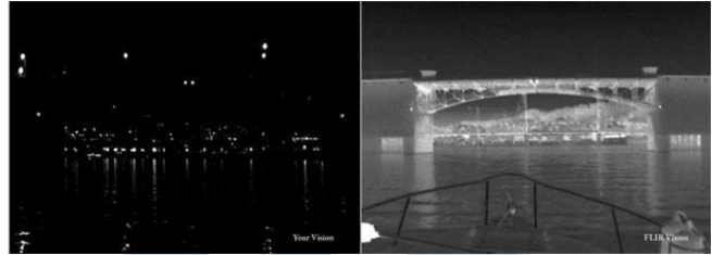
Fig. 216. Naked eye night vision versus thermal imaging using forward looking infrared imaging
