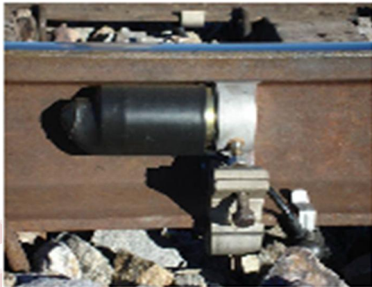
Fig.1 Ultrasonic Broken Rail Detector
