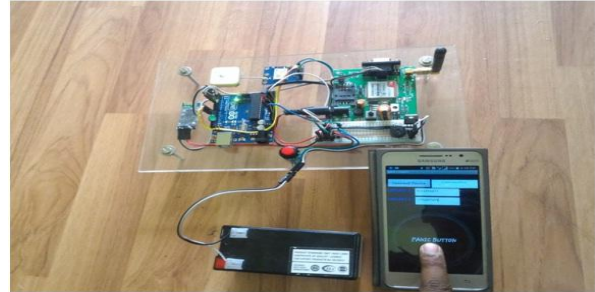
Fig 5: The proposed model operated through an android app
