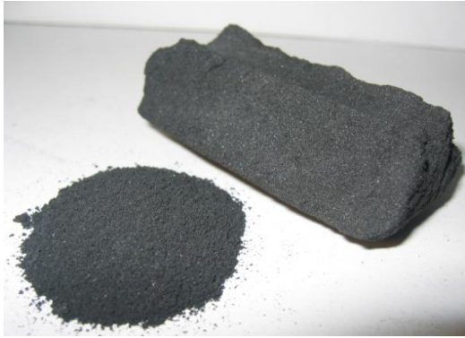
Fig 9 Activated carbon of IV value 1000 that is being used and MBS value about 350
