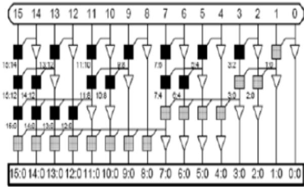
**Fig 4(a): Schematic Wallace tree multiplier**
