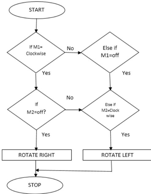
**Fig.4: Flow chart of algorithm to control platform**
