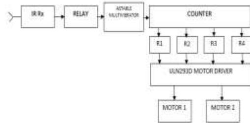
**Fig.6: Robotic Arm Control**
