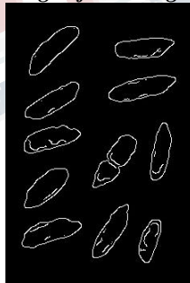
Figure 6 After applying canny edge detection to the pre-processed image
