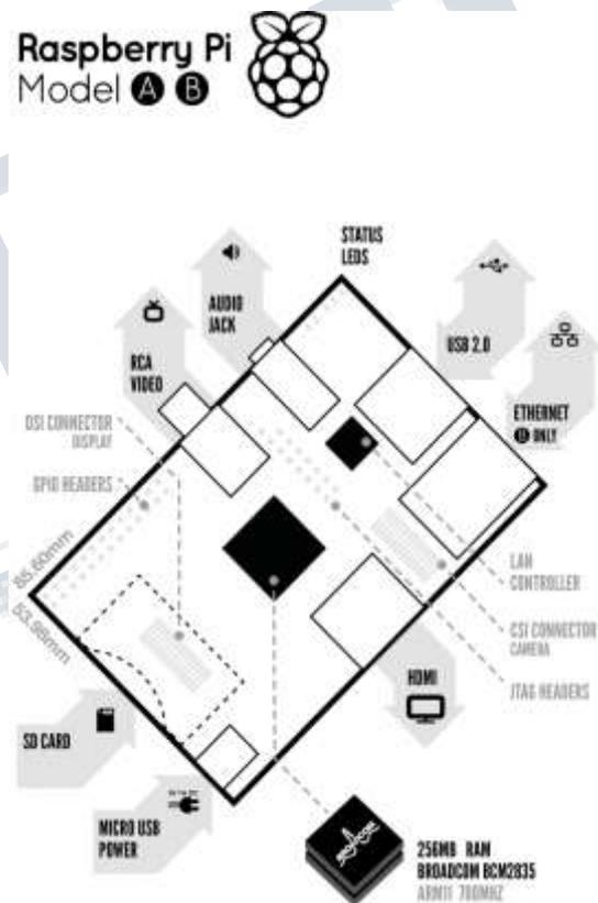
Fig: Raspberry pi 1 model B+
