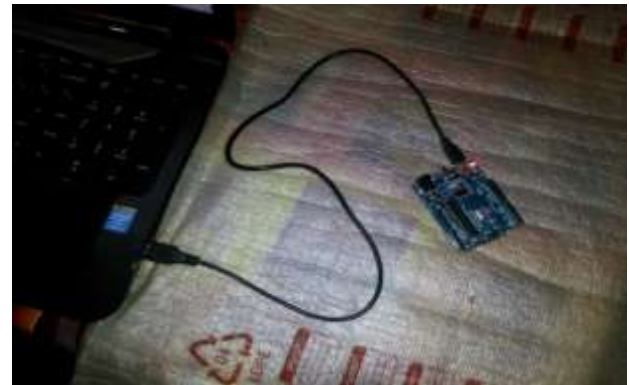
Fig 3: Connecting Arduino Duemilanove to the system through USB port.
