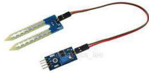
**Fig.6: soil moisture sensor**
