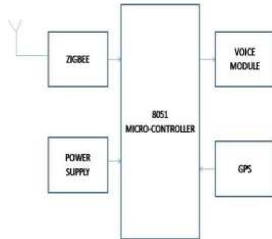
Fig (2) Block Diagram of Receiver Section
