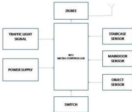
Fig (1) Block Diagram of Transmitter Section
