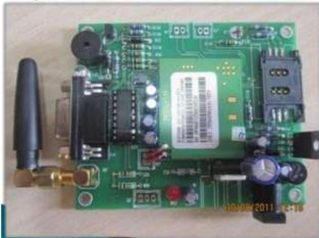
**Fig 2 GSM Module**
