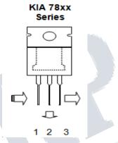
The stabilization of d.c. output is achieved by using the three terminal voltage regulator IC. This regulator IC comes in two flavors: 78xx for positive voltage output and 79xx for negative voltage output. For example 7805 gives +5V output and 7905 gives -5V stabilized output. These regulator ICs have in-built shortcircuit protection and auto-thermal cutout provisions. If the load current is very high the IC needs 'heat sink' to dissipate the internally generated power
