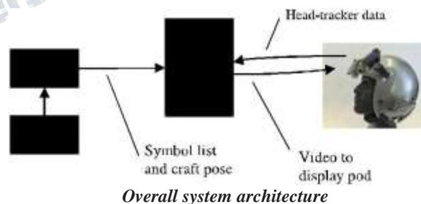
In general for avionics “harmonization” is the process of aligning the axes of various aircraft systems with one another, such as the inertial navigation system, the heads-up-display (HUD), the HMD tracking system reference, sensor pods or targeting pods, and weapons. We developed a variety of tools and methods to align the fiducially constellation with the aircraft axes, or more specifically with the platform INS axes since the INS is the reference frame from which symbol generators are
