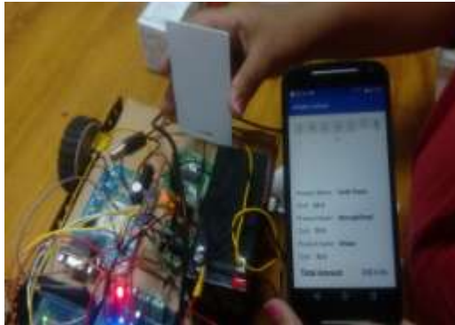
Figure.6: RFID reader with item details and tags.
