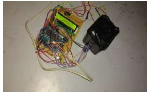
Figure 1. Electronic circuit for color sensing
