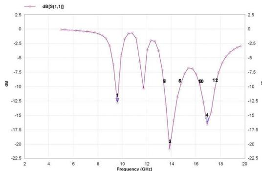
**Figure 2 The return loss of the multiband newly formed fractal shape microstrip antenna for different values of position of R1(x1,y1) and R2(x2,y2) respectively (0.5,3) and (0.5,-3)**
