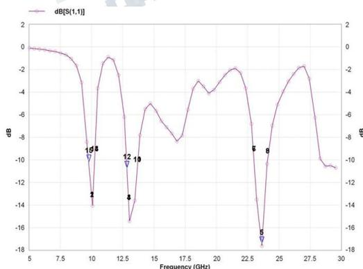
**Figure 4 Return Loss Vs Frequency of Finally Designed**
