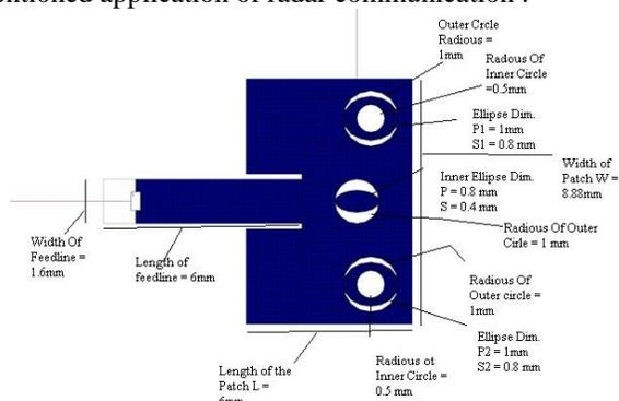
**Figure 3 .Compact Crown Circular Patch Antenna for X, Ku and K Band Applications {position of C1 and C2 are (0.5,3) and (0.5,-3) respectively}**
