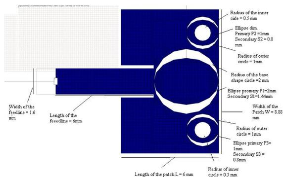
**Figure 1. Compact Crown Circular Fractal antenna for operating on multiband application (Position of the C1 and C2 are (1, 3) and (1,-3) respectively).**
