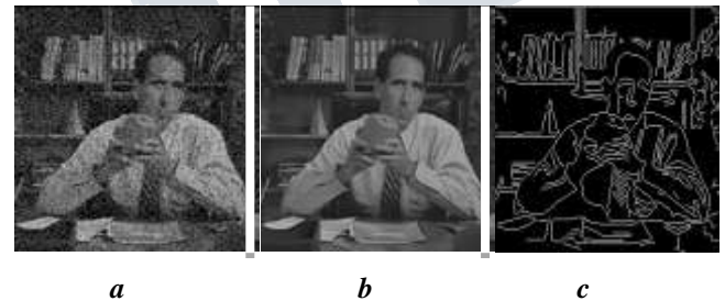
Fig 6: (a) image with noise, (b) histogram output, (c) edge images
