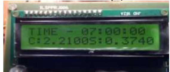
Fig 9: Power consumes & power saves displayed in LCD unit.
