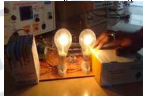
Fig4: Both the street lights are in dim mode.
