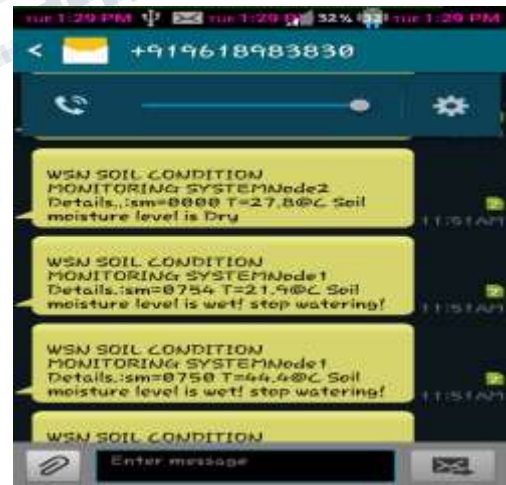
Fig 4.5: SMS notification from the nodes
