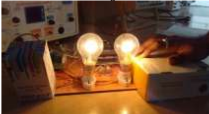
Fig3: Both the street lights are in dim mode.
