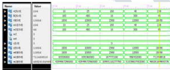
*Fig 4 shows the output of approximate multiplier Architecture for different inputs*
