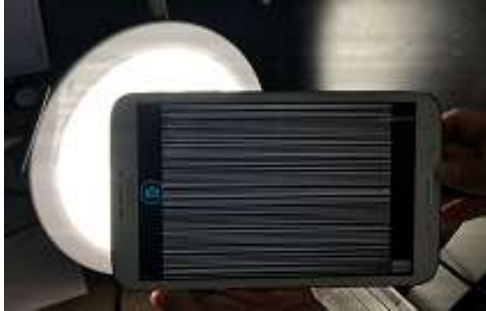
Figure 8: VLC Link – Evaluation Model using Smart Device
