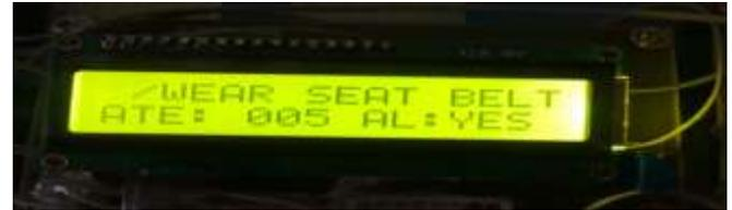
Alcohol consumed. So the bus automatically stopped (LCD displays as AL: YES).
