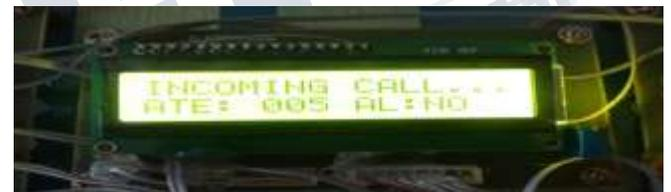
In driving if any incoming call occurred it disconnect within two rings and send message as I'm in driving.
