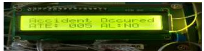
Accident occurred the vibration sensor is activated. This information sends to controller and LCD displays accident occurred and number of persons in the bus. Buzzer will be ON, Then the bus automatically stop.
