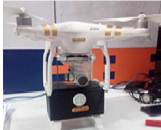
Figure9: Integration of the designed embedded circuit enclosure box with the Quad copter
