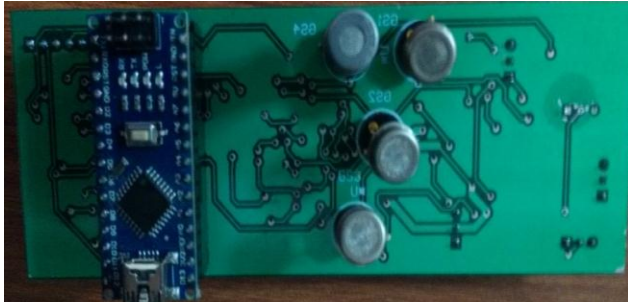
Figure 4: PCB Bottom View
