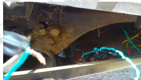
Fig 7: Placement of Arduino and Bluetooth module in vehicle 2(Hero Honda Pleasure)
