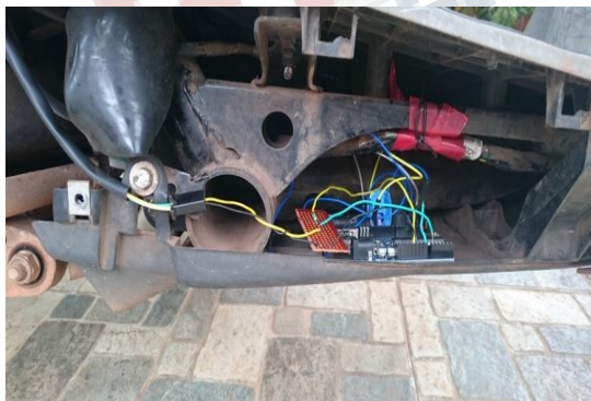
Fig 10: Placement of Arduino and GSM module in the vehicle (Honda Dio)
