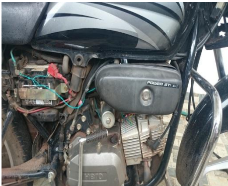
Fig 3: Battery connection for vehicle 1
