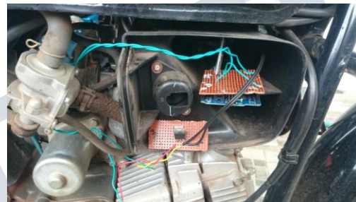
Fig 6: Placement of Arduino and Bluetooth module in vehicle1(Honda Splendor)
