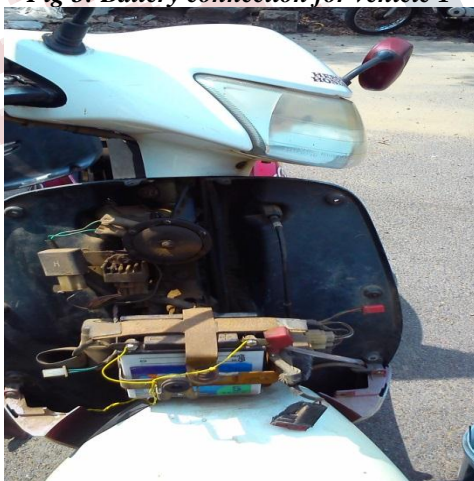
Fig 4: Battery connection for vehicle 2
