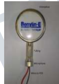
Figure 2: Chestpiece, Tubing and Microphone assembly
