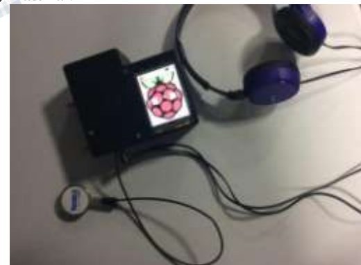
Figure 3: Final assembly with 3D printed casing
