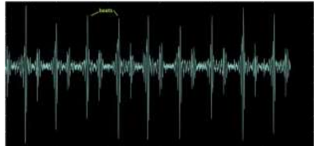
Figure 10: Heart beat signal after processing (with FFT Filtering)
