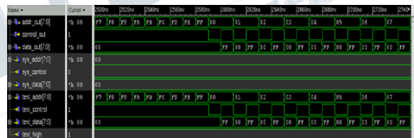
Fig: The output waveform for muxes (MIU)
