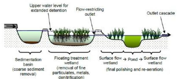
**Figure 2- Conceptual Design of Storm Water Treatment**
