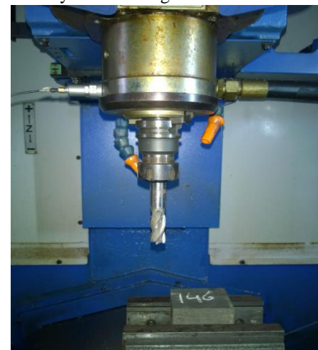
Fig 3. Sensor fixed to the spindle
