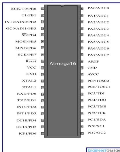
**Fig. 2 Pin diagram of ATmega16**
