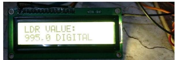
**Fig. 2 (c)** during night time LDR value is maximum
