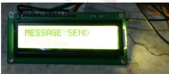
*Fig. 2 (g) message is send through GSM, if vehicle stay on one point more than delay time*
