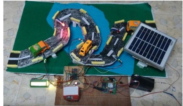
**Fig. 2 (a)** during night time led (lamp) turn ON after detecting vehicle movement
