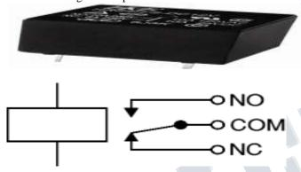
OPERATION: When current flows through the coil, a magnetic field are created around the coil i.e., the coil is energized. This causes the armature to be attracted to the coil. The armature's contact acts like a switch and closes or opens the circuit. When the coil is not energized, a spring pulls the armature to its normal state of open or closed. There are all types of relays for all kinds of applications.
