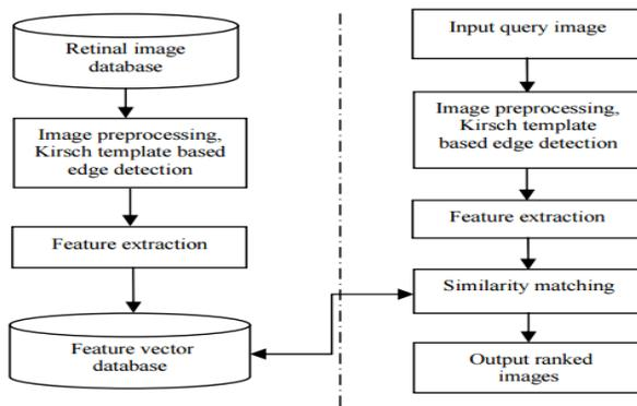
**Fig 1: Content Based Image Retrieval Architecture**
