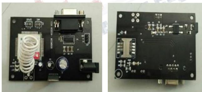
**FIGURE 6. FRONT AND BACK LOOK OF GSM MODULE**
