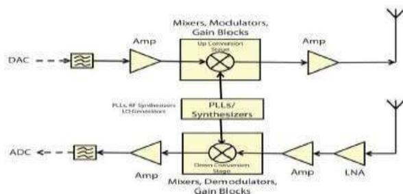
**Fig.4: Block diagram of a typical RF front-end.**
