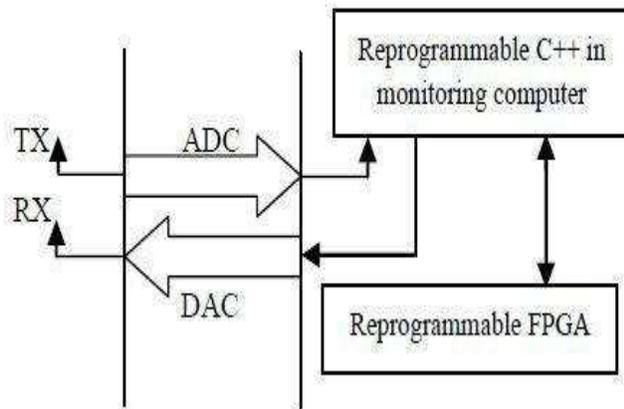
**Fig.2: Block diagram of a Software Defined Radio.**
