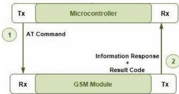
Fig. 3: Connectivity of GSM modem
