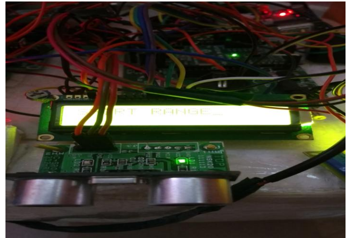
Fig 2- The figure shows the message about the co-ordinates, obstacle detected by the ultrasonic sensor and metal detector
