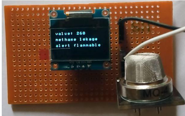
Fig 4: OLED display showing alert message
