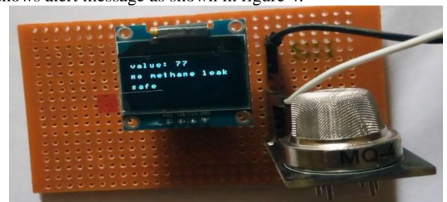
Fig 3: OLED display showing safe message
