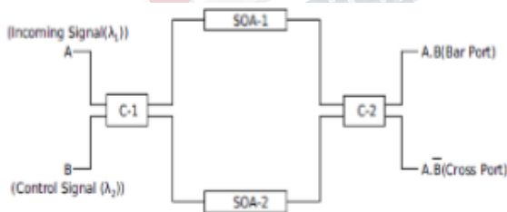
Fig.2. SOA based Mach-Zehnder Interferometer switch [8]
