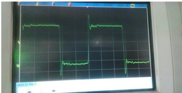
Fig 10. Oscillator square wave output
