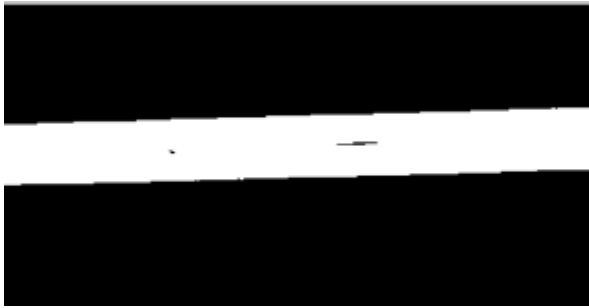
Fig. 5. Image contains edges of pipe and defects
