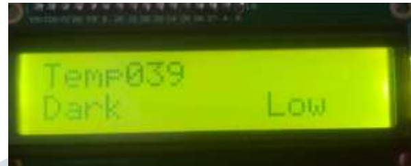
Fig. 10. Image shows temperature(390c), light intensity(dark) and water level(low)
