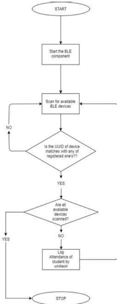
**Fig 6: Flowchart of application at PSoC device.**
