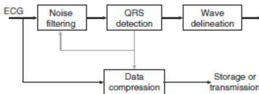
**Figure 2: Block diagram of basic ECG Signal processing**
