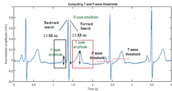
**Figure 6: Formulation of T and P wave search windows and thresholds**
