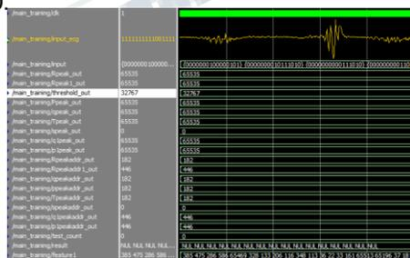
**Figure 10: Simulation result for QRS complex and feature extraction**
