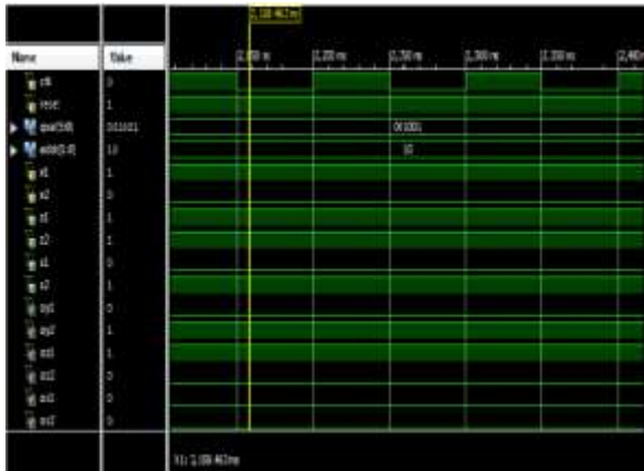
Figure 11. Simulation of the microprogrammable 2 bit signature analyzer
