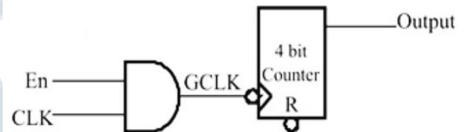
*Fig.2. Clock gating using AND gate Circuit*
