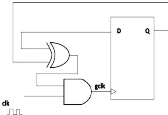
**Fig.4. Clock gated D flip flop**
