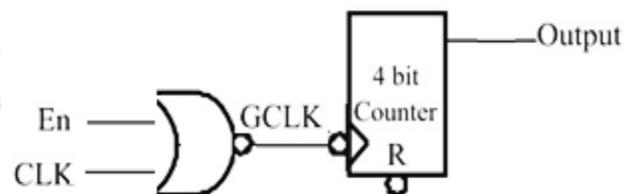
*Fig.3. Clock gating using NOR gate Circuit*
