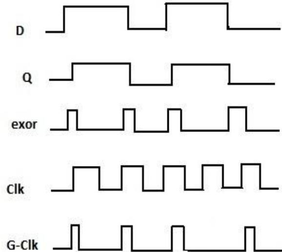
**Fig. 5. Waveform for gated D flip flop**
