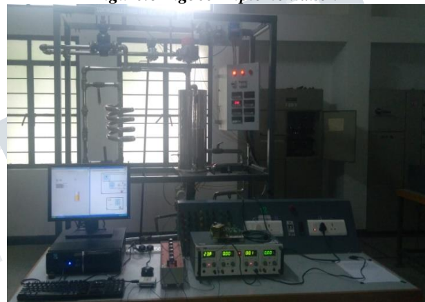
Figure.7 Experimental setup of CSTH Process
