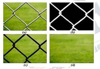
Fig.1(a) Input image with a regular fence, (b) Segmented fence mask, (c) The fence masked image, (d) Restored image from the fence occlusion by using hybrid inpainting algorithm
