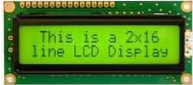
Figure5: 2x16 Line Alphanumeric LCD Display
